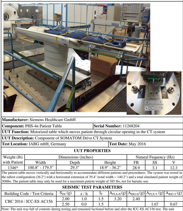
maintained structural integrity during and after the ICC-ES AC156 Test.
