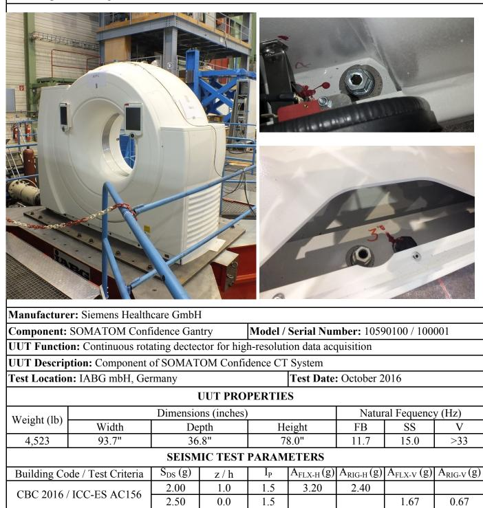
Note: The unit was full of contents during testing and remained fuctional before and after the ICC-ES AC156 test. The unit maintained structural integrity during and after the ICC-ES AC156 Test.
